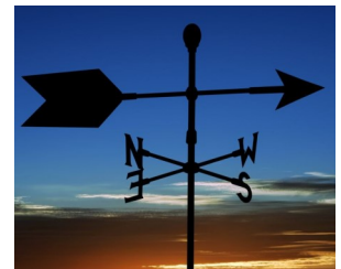
Weather vane— measures the direction the wind is blowing
